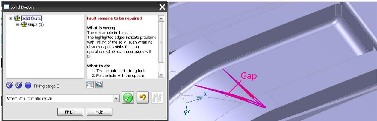
The final inconsistency is caused by a degenerate surface (possibly as a result of a translation error).
