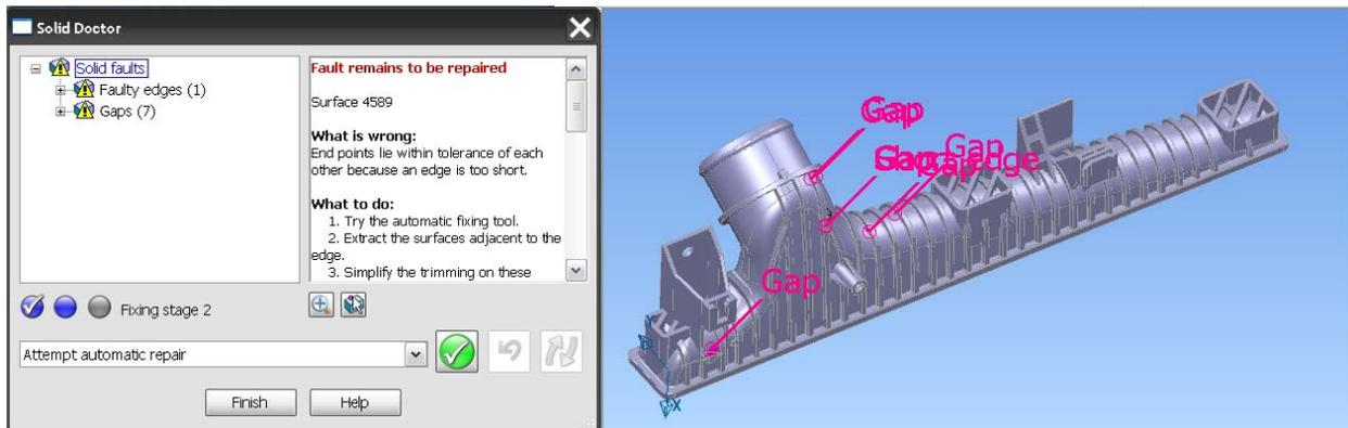
Solid Doctor checks the solid for consistency issues and displays them in an easy to understand tree, and also marks their locations graphically on the model. Issues are divided into separate categories, each of which has an automatic fix and a recommended alternative strategy. The user can select individual issues either from the tree or graphically on-screen. This allows the user to tackle issues in whichever order, and by whatever method, they feel most appropriate.
