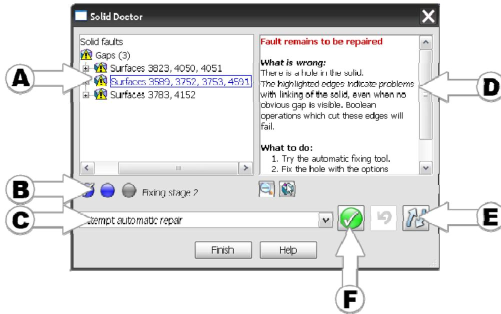
A – Categorized list of consistency issues, displayed as an easy-to-read 'tree', clearly showing which surfaces need further attention. Issues are also highlighted graphically on the model and can be selected either from the tree or in the graphics window. The user may select issues individually, by category, or by normal Windows-style multiple selection (using Ctrl and Shift modifiers).
