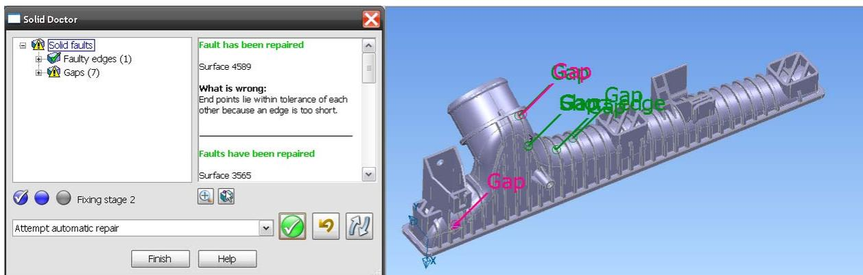
After automatic repair, issues that have been attended to are clearly highlighted, both in the graphics window and the tree, for ease of identification.
